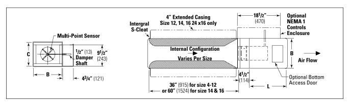
Damper rotation is always clockwise to the open position. An identification mark on the end of the shaft indicates the damper position.
